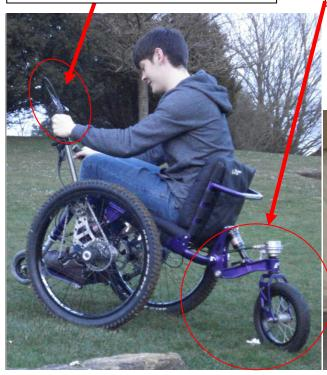
A powerful disk brake is on each wheel. These are operated using a single brake lever to give even braking and easier operation. A simple and patented handbrake mechanism is also incorporated.
