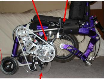
With the wheels removed and the rear wheel folded up, the bash guard protects the gears and disk brakes during transport.
